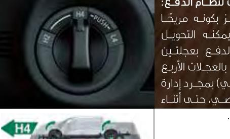
**Part-time transfer:** Highlighting driver-friendly operation, you can switch between 2WD and 4WD by simply turning the dial switch, even while moving.
